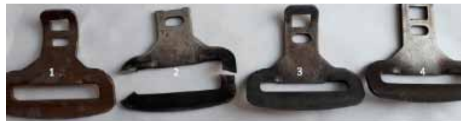
Figure 5. Hardening influence to the mechanical properties. 1 – soft and ductile part without hardening, easily bendable; 2 – hardened part without tempering, really fragile and breaks already applying minor force; 3 – hardened and high temperature tempered, bendable only by applying bigger force; 4 – hardened and tempered with optimum tempering, bendable only slightly and when by applying big force
